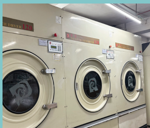
Dryers with Variable Frequency Motors
