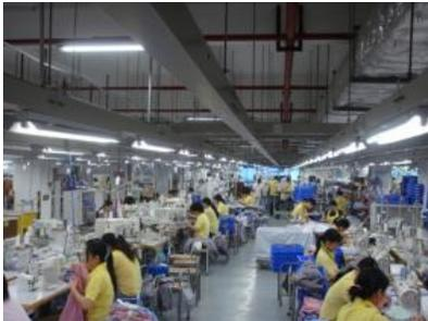
Reflectors are used to increase brightness, and lighting has been installed with independent switches near users.
