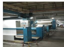
Shrinking machine in printed rib fabric process
